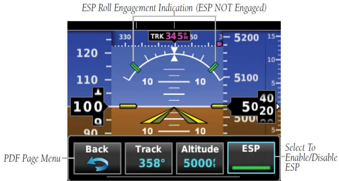
Figure 3-25 AFCS (ESP Enabled)
